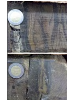
Dark brown sand ripple thin intervals with hydrocarbon impregnation Core 1, Well T.
